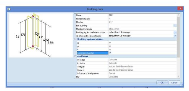
Afterwards, a label will be displayed on beam B17, indicating that this beam consists some buckling data. This buckling data is **Additional data** and can be copied to other members in the structure.
